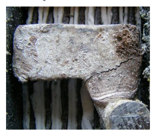
A battery that has failed due to shock and vibration damage cannot be repaired or recovered. It is recommended that you protect your battery by using proper mounting methods with foam. Hard rubber mats such as those found in tool chest drawers offer minimal protection as they do not effectively damp vibration.
